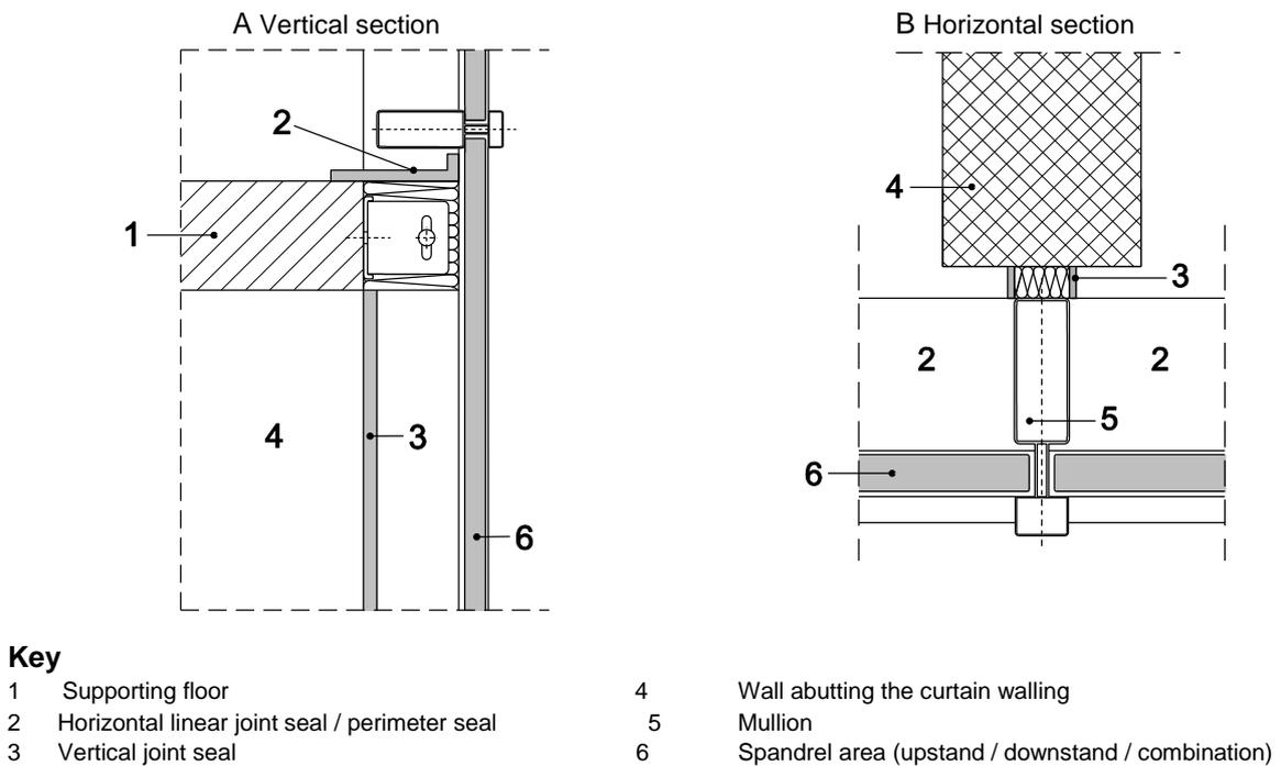
**Figure 2 – Linear joint seals abutting curtain walling**
