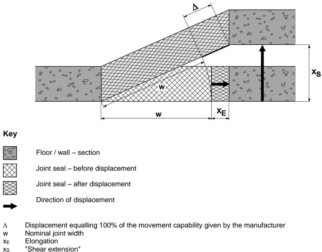
**Figure 16: Test condition with a combination of lateral elongation and shear at the maximum of the nominal width**
