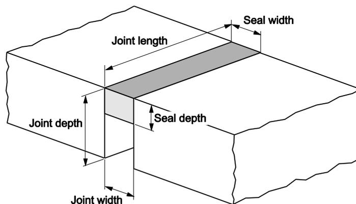
**Figure 3 – Definition of seal depth, joint depth and joint width**
