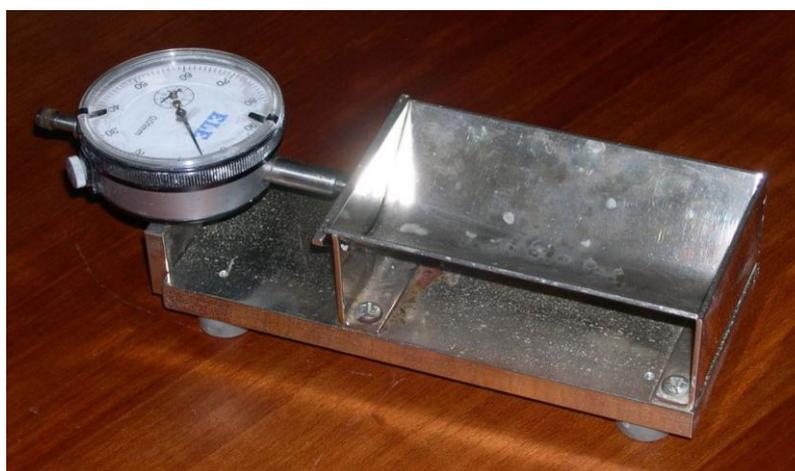
Figure 13 – Extensometer
