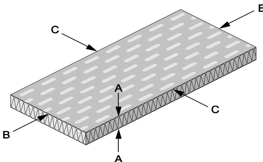
**Figure 4 – Mineral wool – Compression directions**
