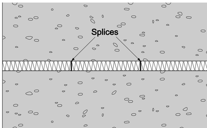
Figure 18 – Mineral wool – Distance between splices
