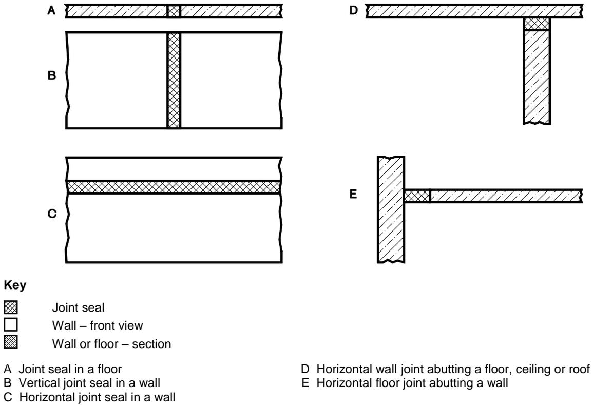
**Figure 1 – Possible orientations of linear joint seals**
