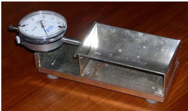
**Figure B.5 – Extensometer**
