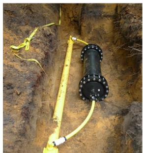
Figure 10 – Test rig for G-gas
