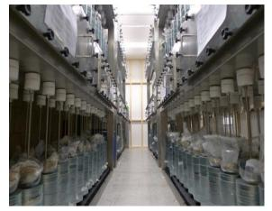
Figure 6 – Full-scale set-up (30 mbar(g)) used to determine the effects of sustainable gases on polymeric materials
