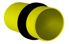
Figure 4 – Set-up for exposing stressed rubber rings to a particular gaseous environment
