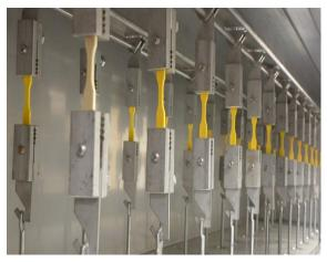
Figure 5 – Constant load experiments on PVC samples
