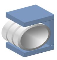
Figure 2 – Principle of a U-clamp test on PE and POM rings
