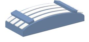
Figure 3 – Principle of a Marbone clamp test on POM tensile test bars
