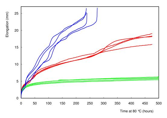
*Figure 3. Slow Peel Tests on joints made in pipes made of resin D (red), resin E (green) and resin F (blue). Each group shows the curves of 4 out of 12 test bars.*
