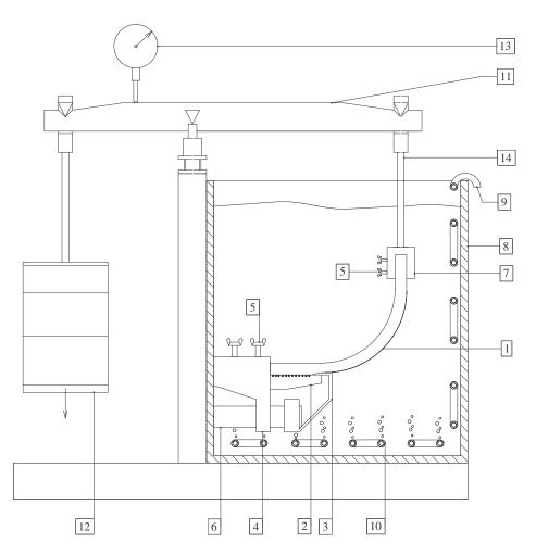
Figure 2. Principle of the Slow Peel Test.
